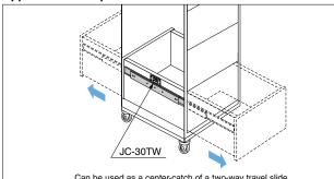
Can be used as a center-catch of a two-way travel slide
