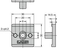
Strike and mouting plate for strike \*Setting of retaingin force: low
